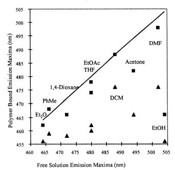
**Figure 7.** Emission maxima of free dansyl monomer vs emission maxima of dansyl monomer polymerized in a 10% cross-linked resin: ▲, MR; ■, JJ.
